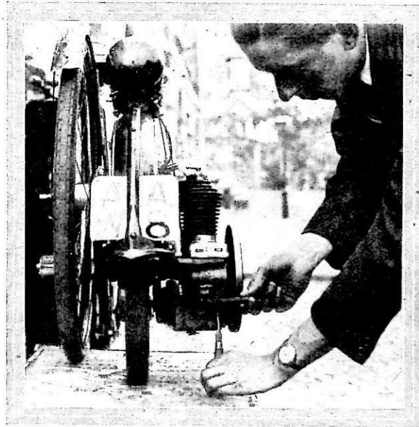
Adjusting the oil screw.
