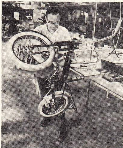
LEFT: An operator is shown fitting the pedal assembly to a Spacemaster.
