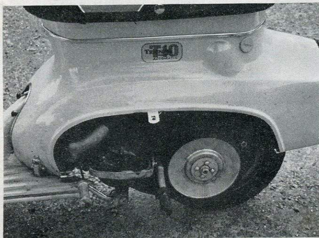
Kickstart is on the left-hand side of the scooter and is simple to operate. Belt drive to the rear wheel sinks deeper into the pulley raising gear ratio with speed.
