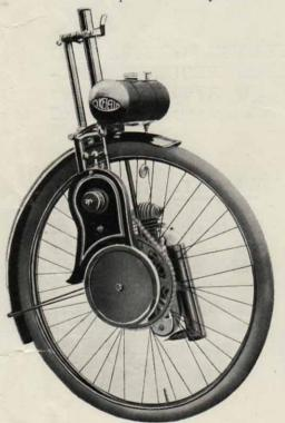
CYKELAIDE, as illustrated, ready with correct size of head tube, to take the place of the front wheel in any make of pedal cycle. 1¼ H.P. Two-Stroke Engine, Automatic Lubrication, Amac Carburetter, Runbaken Magneto, Hand-operated cork-inset Clutch, Girder Spring forks, 28" wheel, without tyre, but complete with all necessary control wires and levers.
