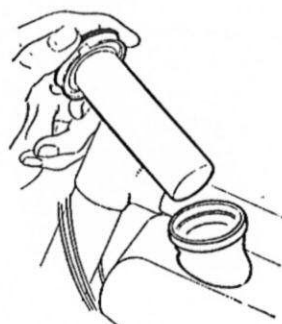
To ensure the correct proportions of oil and petrol, a measure is fitted to the underside of the filler cap. Four measures of oil are mixed with every gallon of petrol.
