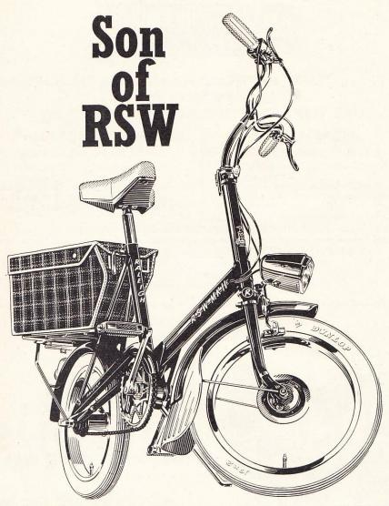
This is the RSW Mk II — new development of the acclaimed RSW 16. Seen in colour by millions of Daily Express readers on November 24th! Differences? Extra frame height. More seat comfort. New handle-bars with self-adjusting twist grip. New S3B rear hub for better braking. And lots of other new features. Price? — only 30½ gns. Cash in on a success — now!
