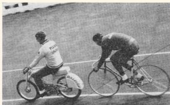
SPECIALLY BUILT BY RALEIGH for the Skol-Six is this prototype "Pacemaker" being tested here by Dutch rider Gerard Koel. Six of these 50 mph machines are being produced at Nottingham for motor-paced events at Earls Court.
