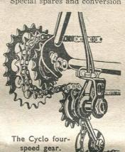
parts for the four-speed gears are featured, as are the company's special rear fork-ends and various types of fitting brackets and rear hubs.
