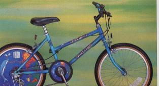
Freedom Shimano 5 speed index gearing with thumbshift control - for fast and accurate gear changing. ■ Semi-raised handlebar for confident control. ■ Anatomical 'Litefoam' saddle for more comfortable riding.
