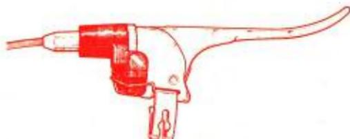
The brake lever automatically adjusts the amount of free play in the cable inner wire by an internal spring actuating a ratchet wheel, which moves the cable adjuster inside the lever hood.
