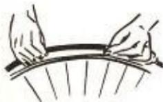
5. Inflate tyre further and seat correctly on rim – true by rolling in proper direction. If there are high or low spots, stretch the tyre where there are high spots – push together where there are low spots. Now fully inflate tyre. It is advisable to allow 12 hours for drying before riding.
