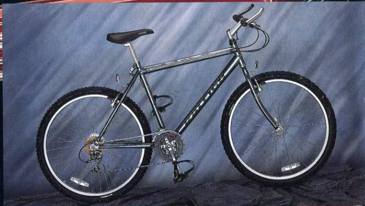
Max Cromo II ■ Super Oversize tig-welded Cromoly frame with oversize, taper-blade Cromoly MTB fork. ■ Shimano STX 21 speed dual index gearing with SRT 300i gripshift system - quick and responsive split grip rotational shifting for improved control. ■ Alloy rims and Shimano Alivio hubs - lighter wheels offering improved handling. ■ Maxxis 2.1" skinwall off road tyres - traction at the rear, steerability at the front. ■ Colour: Gunmetal Mirror. ■ Frame sizes: 16½", 18", 20", 22".
