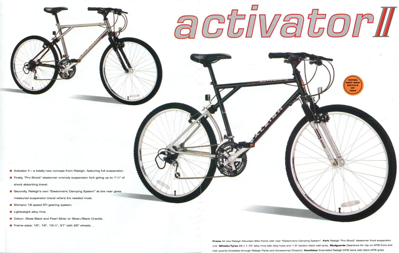
unit. Wheels/Tyres 26 x 1.75" alloy rims with alloy hubs and 1.9" section black wall tyres. Mudguards Clearance for clip on MTB front and rear guards (Available through Raleigh Parts and Accessories Division). Handlebar Enamelled Raleigh MTB bend with black MTB grips.
