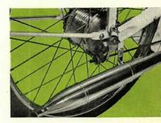
Front and rear axles 11 mm in diameter. Wheels quickly removable.
