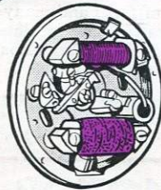
ADVANCED DESIGN STATOR PLATE, EASILY ACCESSIBLE CONTACT BREAKER POINTS.
