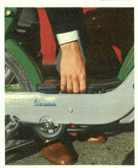
To disengage the engine is simplicity itself. Simply press this button and pedal away. The Ciao instantly becomes a comfortable and smooth running bicycle.
