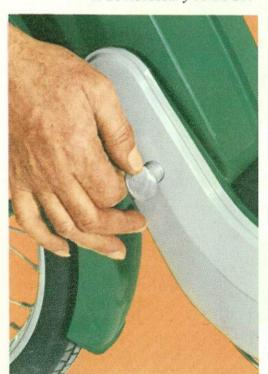
An ingenious carrying handle has been built into the central floorboard. The Ciao can be easily lifted and carried for short distances.
