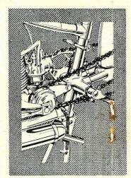
Unique combined casting for bottom bracket with Nylon bearings, rubber bushed engine mountings and strong bipod stands.
