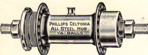
No. 40.—Celtonia Rear Hub. 1\frac{1}{2} " Chain line. Without Gear Case Clearance. Screwed one side only for Cog and Lock Nut or Free Wheel. Flatted for use in \frac{5}{16} " Quick Release Fork Ends.
