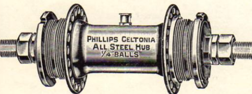
No. 43.—Celtonia Rear Racing Hub. 1\frac{1}{2} " Chain line. Without Gear Case Clearance Screwed both sides to take Cog and Lock Nut or Free Wheel. Flatted for use in \frac{5}{16} " Quick Release Fork Ends.
