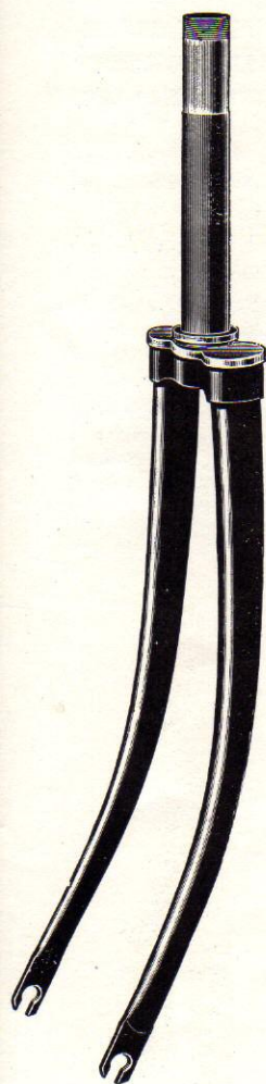
↑ No. 213. Flat Front Fork. With plated Top Plate and Crown Race. Columns 1" dia. Reduced at top to \frac{31}{32} " & screwed 30T for Ball Head Clip as standard. Expander Head 1" × 26T sup- plied to order.
