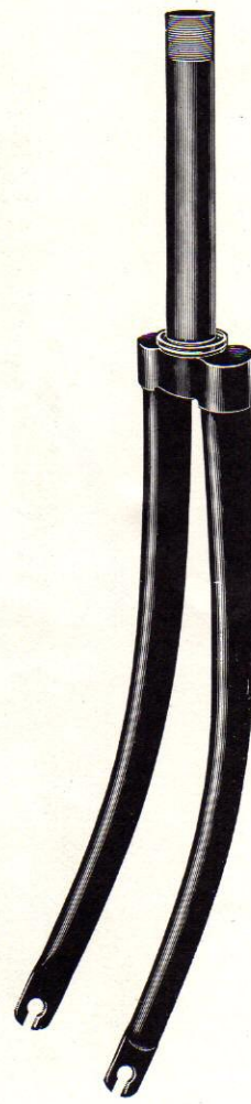
↑ No. 255. Carrier Pattern Front Fork. Constructed from extra heavy gauge material throughout. Columns 1" dia. Screwed 1" × 26T for Expander Head fittings as standard.
