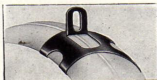
View of Rear Seat Stay Clip for Horizontal Bolt Fastening, as supplied with Models Nos. 269, 272, 279, 282.
