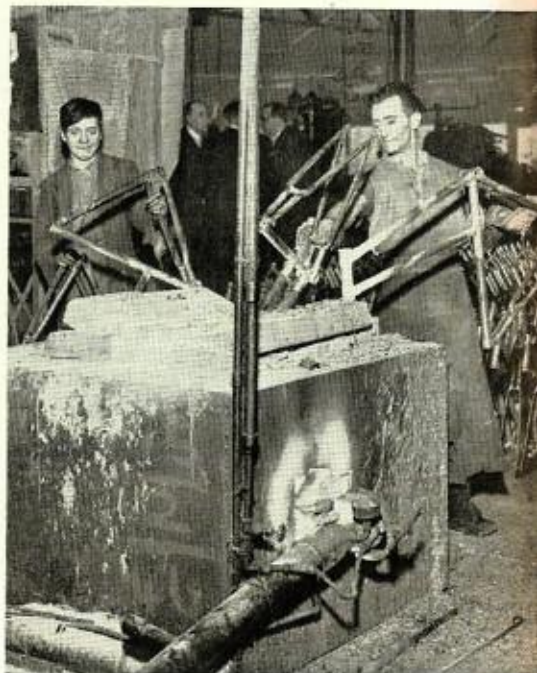
Jigs ensure accuracy when tapping out bottom brackets
