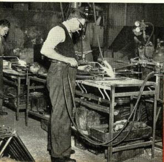
Jig welding rear stays to seat lugs
