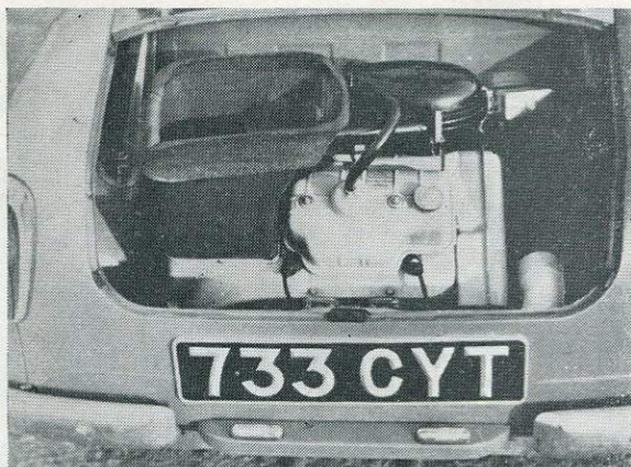
Rear engine compact layout
