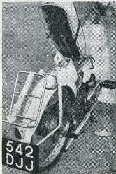
The scooter-type lift-up seat (left) gives access to pump and compact tool box. The plate on the ground is the carburettor cover, held in place by one screw. Carrier is an extra
