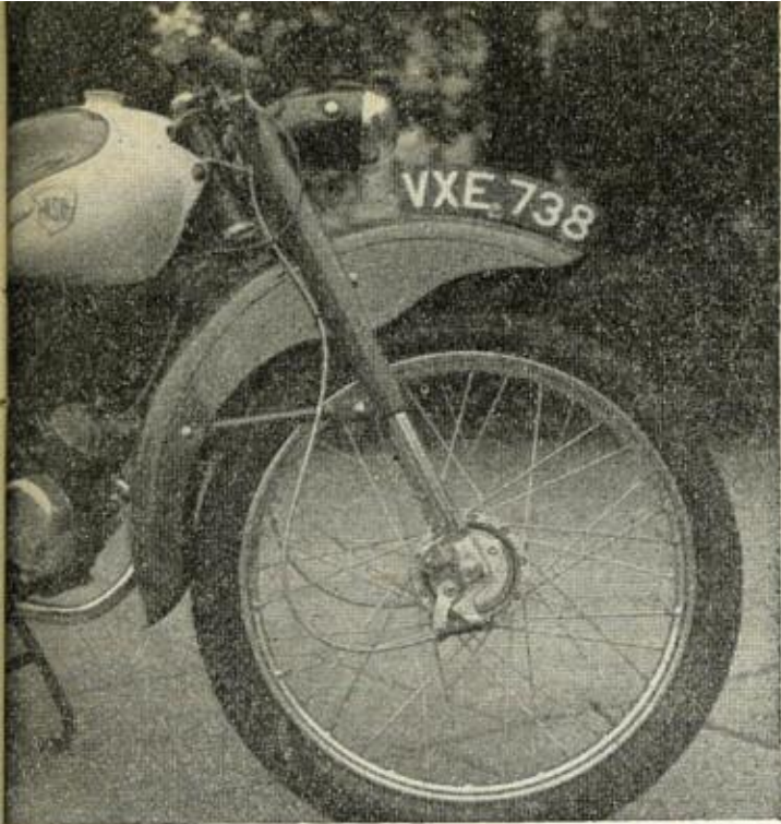
The front end of the CAVALLINO, showing the new telescopic forks.
