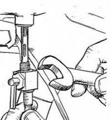
Empty out all but a small amount of petrol from the tank prior to removing the tap and filter; the remaining fuel will serve to swill out the sludge in the tank, requiring only a small amount of clean petrol to complete the job. When unscrewing the tap, the lever should point downwards.
