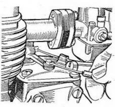
5 Before the gear-change cables can be disconnected, it is necessary to loosen the adjusters at the handlebar twist-grip. This done, slip the two cable nipples from their respective arms on the gear box cover.
