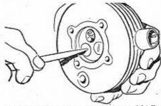
Reseat the valves if necessary with fine grading paste, applying a steady rotary movement with a screwdriver fitted into the slots in the valve crowns. When both valve face and seat are shiny and unmarked, wash thoroughly with petrol to remove all traces of paste. Remove the carbon deposits from the cylinder head and piston with a soft metal implement in the normal way. The cleaner these surfaces, the better the engine's efficiency.
