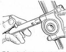
Supporting the engine with one hand under the crankcase, loosen the engine mounting brackets. These are secured by four bolts, which should be loosened in a uniform manner to relieve the stress evenly.
