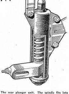
The rear plunger unit. The spindle fits into the aperture in the pivoted horizontal arm. The chain adjuster is seen at the end of this arm, where it is permanently fitted. At the top of the unit is located the grease nipple.
