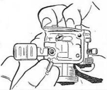
8 The plastic float is hinged on an openended spigot and will slide aff, disengaging float needle at the same time. The the float needle at the same time. The needle is triangular and is grooved at the top to fit into the float.
