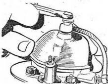
Remove the valve cover after disconnecting the oil feed pipe at both ends to avoid straining. Washers, screws and oil seal should be put aside carefully.
