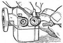
Next remove the banjo union, which is at 5 Next remove the pariso union, and the float the point where the fuel enters the float Soak this also.
