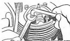
The toppets screw in to the rocker erms and ore secured by lock nuts. Thus they can be screwed in or out to reduce or increase clearance. When adjustment is complete, tighten the lock nut securely.
