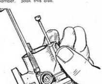
The float chamber is slung neatly below 6 the carburetter body itself, and is removed by unscrewing these two long screws.
