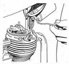
8 Lower the engine carefully on to a box or other support, taking care to avoid strain on the electric cables which lead from the engine up to the headlamp. There is no real need to disconnect these cables, but if necessary, this can be done at the joints. When replacing the engine, the same procedure, in reverse, should be followed. A point to note is that the spring tensioner should be connected before the engine mounting brackets are secured.
