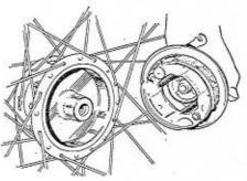
Wash out the drums with petrol, and apply high melting point grease sparingly to the bearings and the brake operating com. On no account should grease touch the linings.
