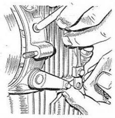
4 Disconnect the clutch cable by lifting the clutch operating lever and slipping the cable end from the nipple here. The length of the clutch cable can be adjusted at this point,
