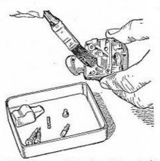
When completely dismontled, soak the 11 carburetter unit and the components in clean petrol and clean with a stiff bristle brush.
