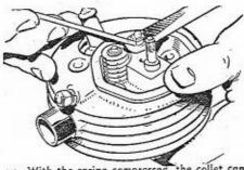
With the spring compressed, the collet can be pushed down the valve stem to expose the small circlip which fits into a groove near the upper end of the stem. Remove this circlip. When opened up slightly, the collet will slide off the stem. Release the spring and remove the valve.
