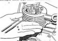
4 On the top of each valve is a small cap; place these, together with the push rods, in a box or tin, marking each either left or right, to ensure that they are replaced in the correct order.
