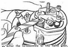
After the re-assembly of the take gear, warm up the engine before checking the tappet clearance with a feeler gauge. The clearance should be 5 thou.
