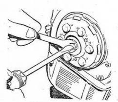
The tap is dismantled by unscrewing the hexagonal nut behind the lever. Sludge may accumulate behind the spring, and this should be cleaned accordingly. When the valve is replaced, the two points arrowed should coincide.
