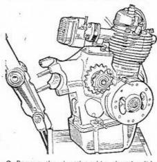
6 Remove the throttle coble, throttle slide, etc., from the carburetter and disconnect the earthing wire which is anchored by the offside valve cover screw. Finally disconnect the upper spring suspension which joins the cylinder in front of the valve cover (the valve cover has been removed in our drawing.
