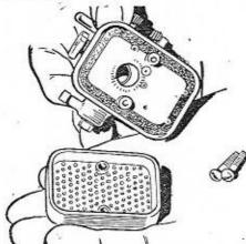
4 Remove the air filter (two screws) and soak it in petrol. Carefully remove the cork seal from the carburetter body.
