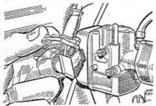
Before starting to dismantle the carburetter wash down the complete unit with Then remove the throttle slide and disconnect from the cable end. Disengage the throttle cable by pushing the nipple down and sideways.
