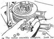
3 The rocker assembly complete. Look for signs of wear in the tappets and the rocker caps. Tappets can be replaced cheaply, but damaged rocker caps mean new rockers.
