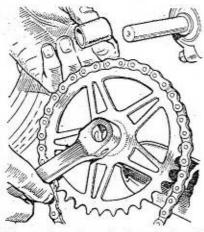
Remove the cotter pins from both pedal cranks and slide the chainwheel off the spindle, slipping the pedalling chain from the sprocket at the same time.
