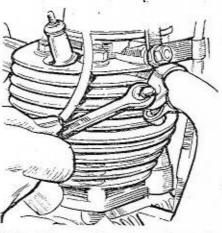
3 Next disconnect the exhaust pipe at the cylinder by loosening the clamp. The silencer is also secured by a bracket at the bottom of the crankcase.
