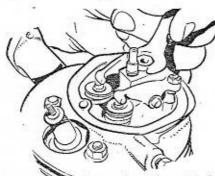
Unscrew the hexagonal securing nut to free the rocker assembly. Take care not to misplace the small brass sleeve on the oil feed stub.
