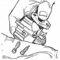
Take care when unscrewing the jets as the Soft bross will damage easily. Obstructions in the jets should be cleared with bristle rather than wire, which may enlarge the
