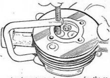
A valve extractor is necessary for the removal of the valves and springs. Place the open end of the extractor over the valve spring and the "driving" and on the valve crown. Avoid scretching the crown.
