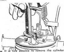
bead. Use a tubular spanner, loosening the nuts gradually in diagonal order to relieve the stress uniformly. When the head is off, check the gasket on the lip of the barrel for signs of gas leak. A new gasket costs a matter of pence. Remove also the rubber oil seels from the push rod guides.
