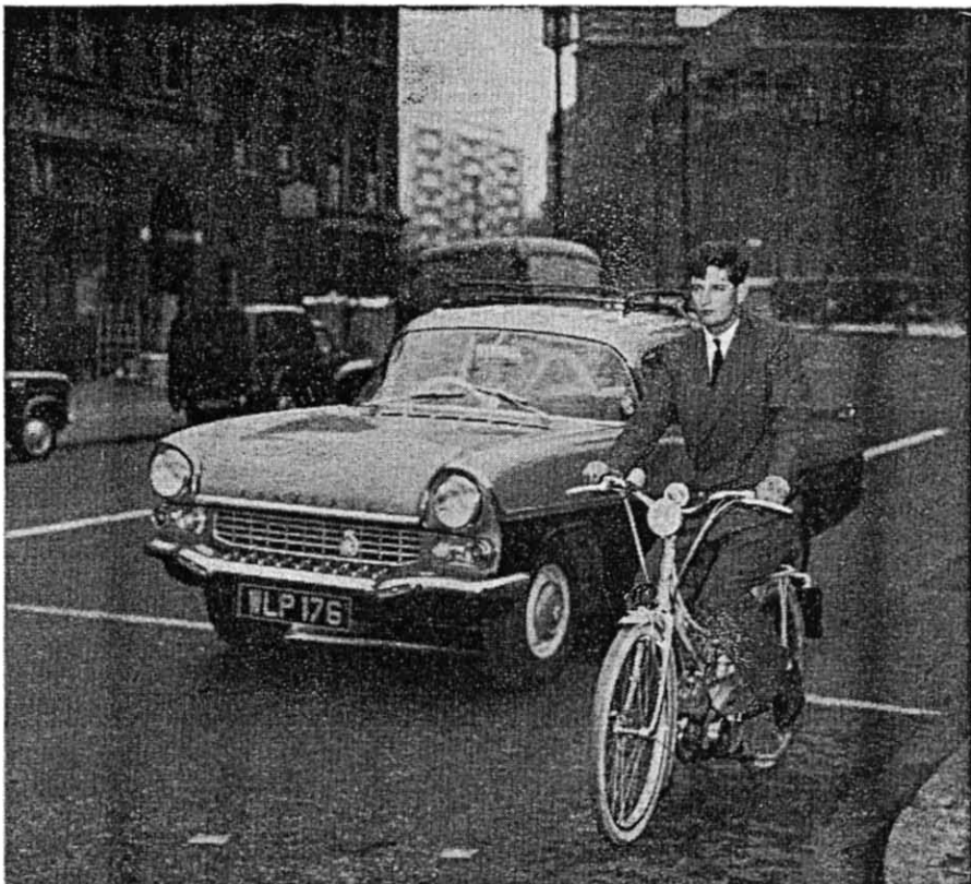
Probably the easiest motorised vehicle on the market to drive, the Mobylette, with its centrifugally operated automatic clutch is ideal for congested city traffic. With a little energetic pedalling to help the willing 50 c.c. engine, remarkably rapid getaways can be made from traffic light stops!
