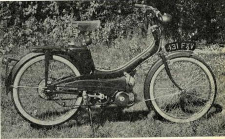
and there is a rear carrier designed to take really substantial loads if required.
