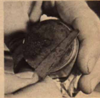
18. Flat topped pistons are best cleaned with a feeler gauge, but make sure to hold the gauge flat and don't scratch the top.
