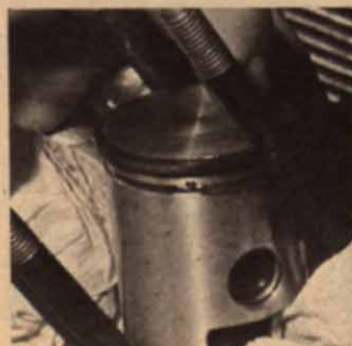
16. Mark the front of the piston before taking it off the con-rod. As a double check notice the position of the ring pegs.
