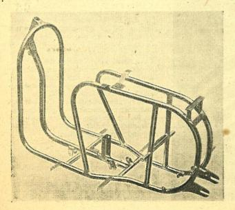
The main frame is constructed from lin × 16gauge tubing and during development it was subjected to five months' testing in a research laboratory
