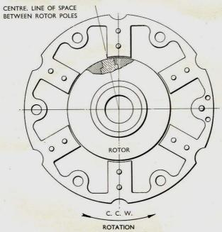
The sketch illustrates the correct position of rotor pole in relation to stator pole when contacts are just opening.
