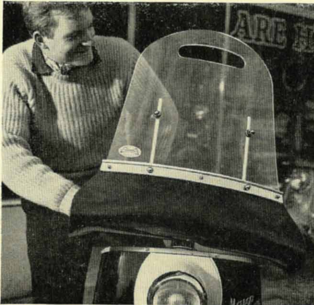
Windscreen made from 'Perspex' acrylic sheet and fairing made from 'Darvic' rigid p.v.c. by Stratford Auto Components Ltd., Masons Road, Stratford-upon-Avon, for the Maicoletta Scooter.
