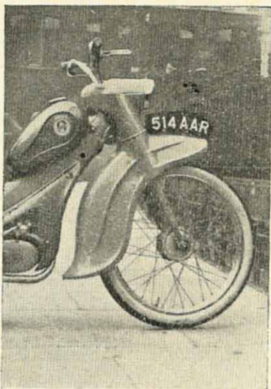
The cowled-in headlamp with adjustable beams is streamlined into the handsome and massive front mudguard.
