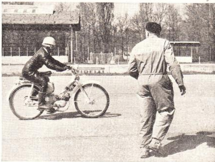
The Lambretta concern have just finished an observed test at Monza with a 48 c.c. cyclomotor which completed 1,433 laps (6,058 km.) at an average speed of 60.5 k.p.h. Here the machine is seen on the circuit.
