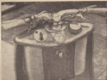
Dashboard layout of the Kieft scooter. The handlebar is a polished light-alloy casting
