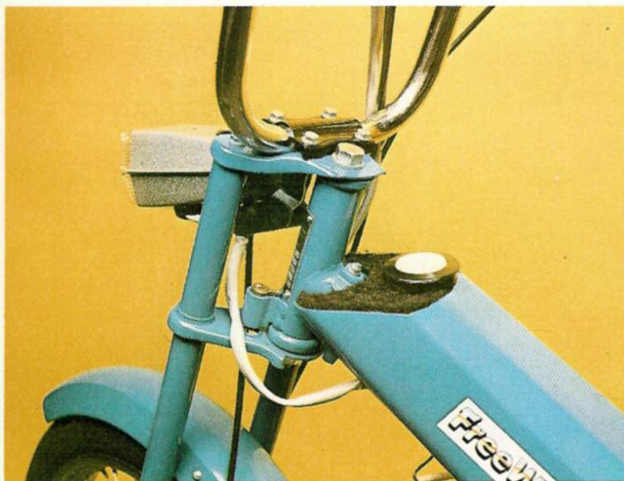
The Jawa's speedo is set in the headlamp shell. Round the tank filler is the felt pad of dubious value
