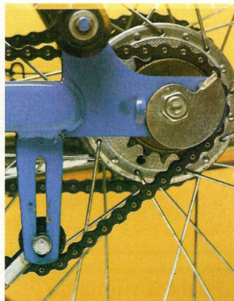
The rear chains of the Jawa needed very frequent attention, but fortunately the adjustment is easy
