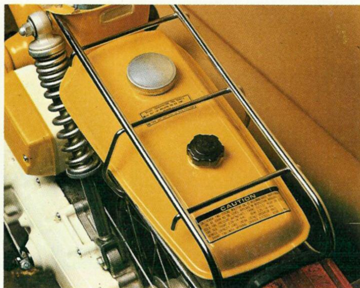
The Honda's fuel tank is neat looking but not very large. The black plug at the rear is for 2-stroke oil
