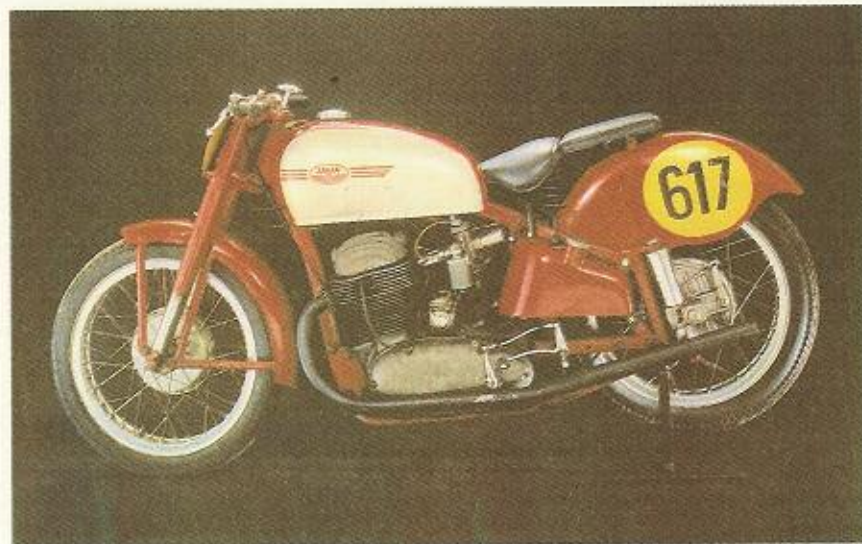
JAWA 500 Racer ● Four stroke air-cooled OHC twin cylinder ● Displacement 488 cc (bore and stroke 65×73.6 mm) ● Engine power about 30 kW ● Camshaft drive by vertical shaft ● Lubrication by pump from auxiliary tank located on the frame ahead of the rear mudguard ● Four-speed gearbox in unit with the engine ● Multiplate clutch in oil bath ● Simple, closed in the rear bifurcating frame made with square steel sections ● Rear wheel slider type suspension ● Telescopic front fork ● Maximum speed 190 km p.h. ● Fuel consumption not indicated
