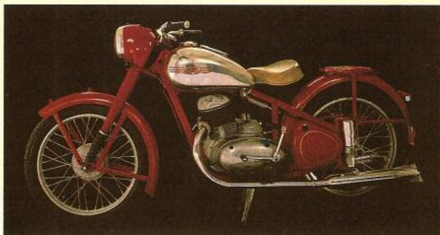
JAWA 250 — Springer • Two stroke air-cooled single cylinder • Displacement 248.5 cc (bore and stroke 65×75 mm) • Engine power 6.6 kW at 4000 r.p.m. • Four-speed gearbox with foot control in unit with engine • Multiple clutch in oil bath automatically disengaged by gearchange pedal movement • Simple closed frame bifurcating at the rear, made with square steel sections • Rear wheel vertical slider type suspension • Telescopic front fork • Weight 115 kg • Maximum speed 100 km p.h. • Average fuel consumption 3 litres per 100 km
