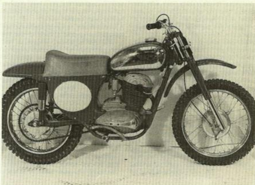
A motocross twofifty — a four stroke engine mounted on a two stroke engine crankcase
