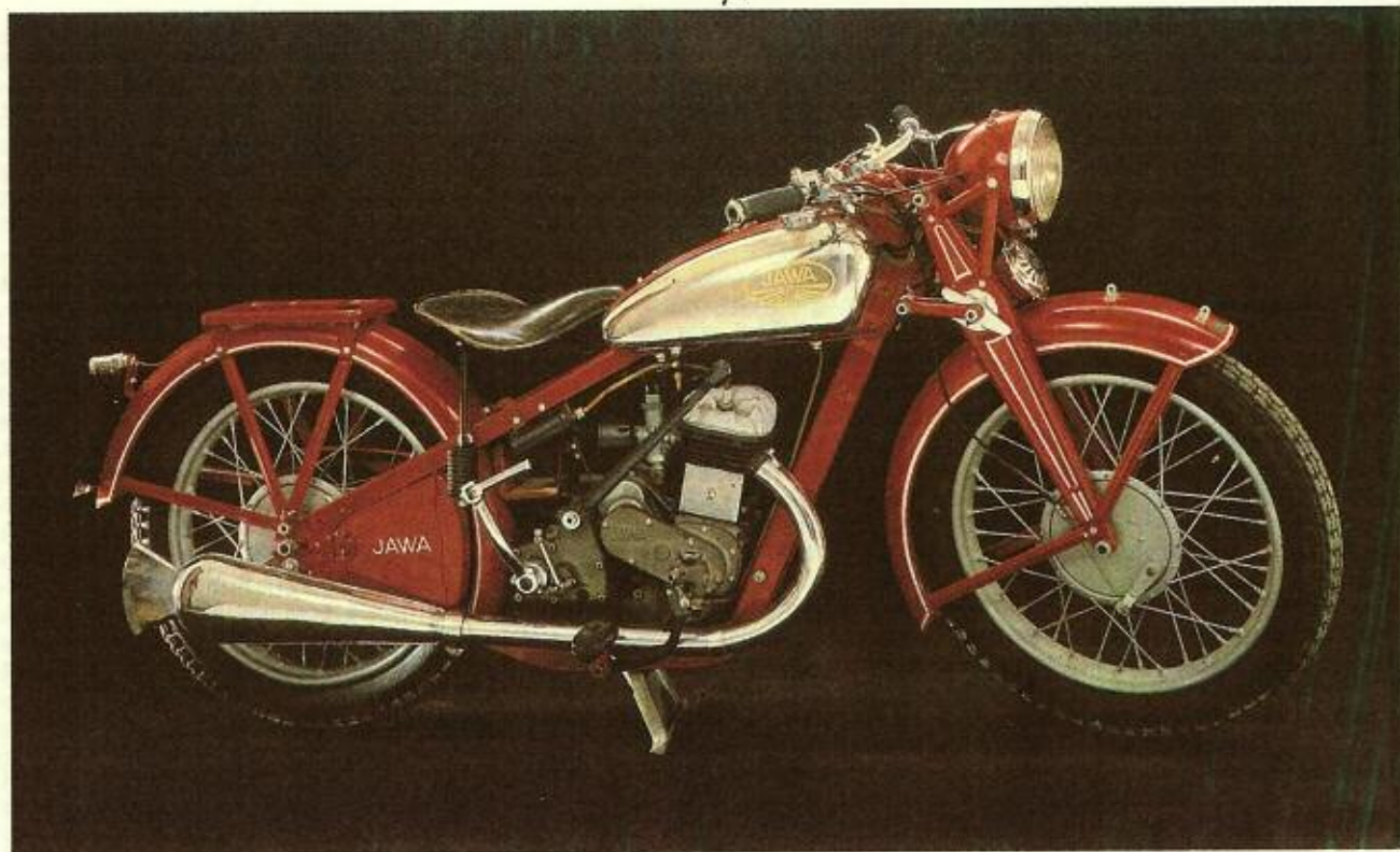
JAWA 350 SV • Four stroke air-cooled SV single cylinder • Displacement 346 cc (bore and stroke 70×90 mm) • Engine power 8.8 kW • Compression ratio 5 to 1 • Oil pump lubrication with oil amount regulation • Separate four-speed gearbox with hand control • Closed duplex frame made with stamped steel sections • Rigid rear wheel suspension • Parallelogram front fork with coil spring suspension • Weight 125 kg • Maximum speed 100 km p.h. • Average fuel consumption 3 to 3.5 litres per 100 km
