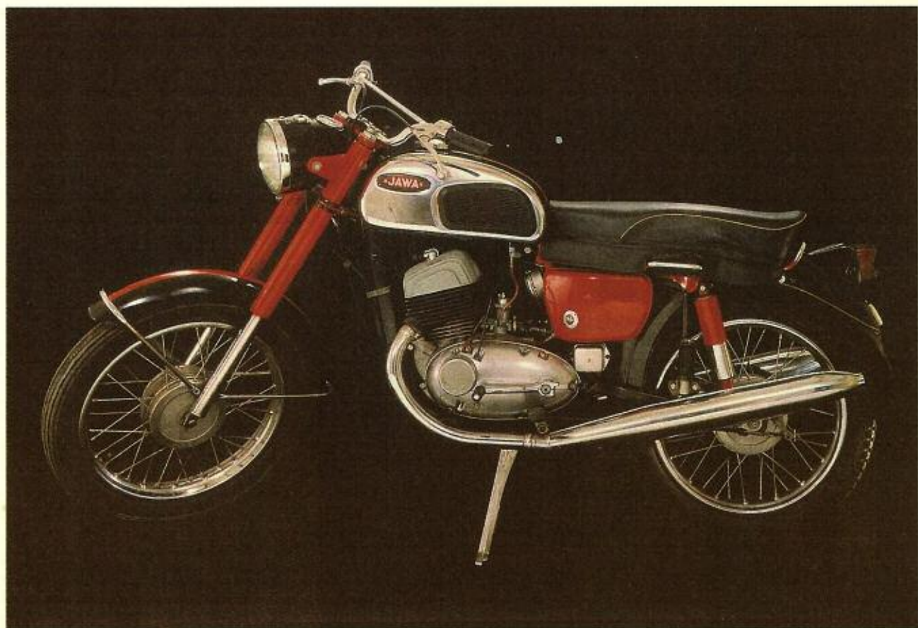
JAWA 350 Californian, Model 362 • Two stroke air-cooled twin cylinder • Displacement 343.4 cc (bore and stroke 58×65 mm) • Engine power 16.9 kW at 5000 r.p.m. • Compression ratio 9.2 to 1 • JAWA Oil Master forced feed lubrication • Four-speed gearbox with multiplate clutch in oil bath • Simple closed frame made with square steel sections • Pivoted rear fork with two oil damped suspension units • Telescopic front fork • Weight 145 kg • Maximum speed 130 km p.h. • Average fuel consumption 4 litres per 100 km.
