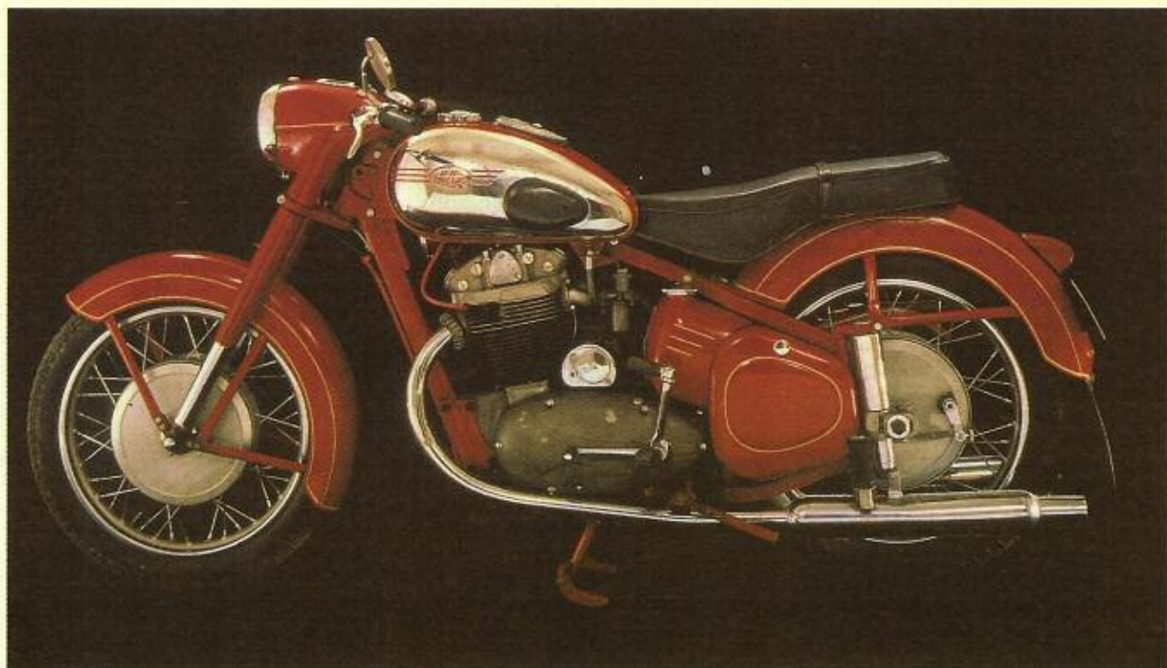
JAWA 500 OHC ● Four stroke air-cooled OHC twin cylinder ● Displacement 488 cc (bore and stroke 65×73.6 mm) ● Engine power 19.1 kW at 5500 r.p.m. ● Compression ratio 7 to 1 ● Vertical shaft camshaft drive ● Lubrication by three-way pump located on the frame ahead of the rear mudguard ● Four-speed gearbox in unit with engine ● Multiplate clutch in oil bath, automatically disengaged by gear pedal movement ● Simple closed in the rear bifurcating frame made with square steel sections ● Slider type rear wheel suspension ● Telescopic front fork ● Weight 156 kg ● Maximum speed 145 km p.h. ● Average fuel consumption 3.5 to 4 litres per 100 km
