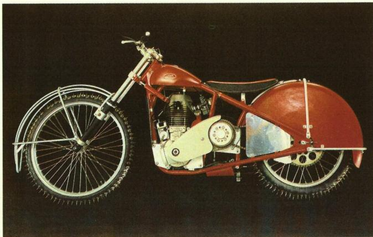
JAWA 500, Model 893 ● Four stroke air-cooled OHC single cylinder ● Displacement 496 cc (bore and stroke 85×87 mm) ● Engine power 42 kW at 8,500 r.p.m. ● Compression ratio 14 to 1 ● Two-valve cylinder head ● Total loss lubrication by double pump ● Oil tank situated aft of the engine ● Multiplate dry clutch ● Two-speed gearbox with foot control ● Simple closed frame made with steel tubes ● Rear wheel without spring suspension ● Telescopic front fork ● Maximum speed and fuel consumption not indicated
