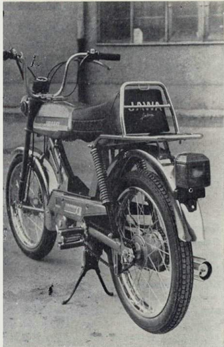
The Babetta Sports is equipped with a tail lamp with brake light and with a relatively robust luggage carrier (picture on the left). The picture on the right is a close-up of the saddle which offers enough comfort
