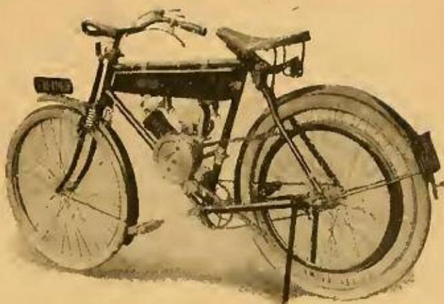
The J.E.S. lightweight motor cycle is on pedal cycle lines, but fitted with the motor attachment and spring forks.
