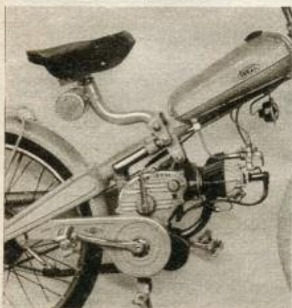
Itom Ideal 48 c.c. with pivoted, spring-controlled saddle tube
