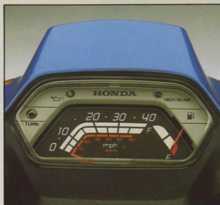
Comprehensive instrumentation with fuel gauge, speedometer, milometer, turn signal indicator lights, oil level and high beam lights.
