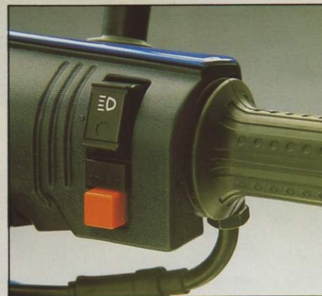
The right handle bar with electric start button, throttle control, front brake lever and light switch.
