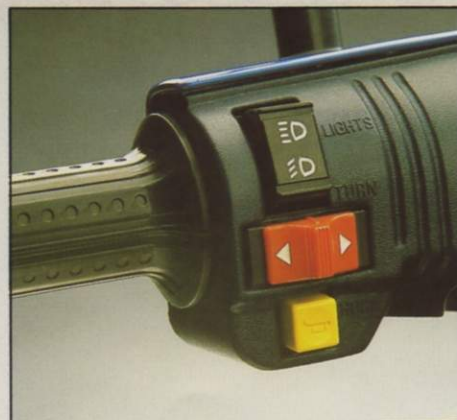
The left handle bar with easy to operate switch gear, rear brake lever, horn, lights and indicator switch.
