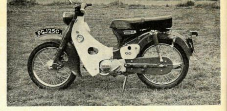
return change. The wet, multiple plate clutch is fully automatic. Fuel tank capacity is claimed to be 1.2 Imperial gallons with engine oil capacity at 1.6 Imperial pints.
