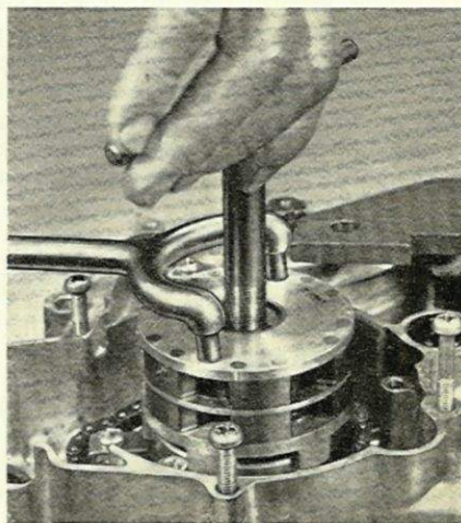
Extracting rotor, using special extractor tool (C102)
