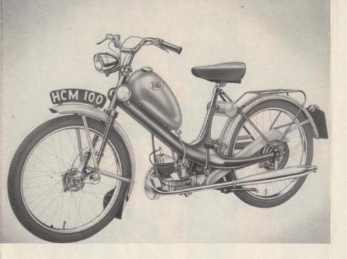
**ENGINE.** 49 c.c. Two-stroke Engine, bore 42 m.m., stroke 35.5 m.m. An "over-square" engine on the most modern lines with ample port areas laid out particularly for good pulling power at average speeds.
