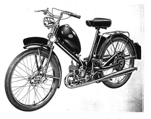
**ENGINE.** 49 c.c. Two-stroke Engine, bore 42 m.m., stroke 35.5 m.m. An "over-square" engine on the most modern lines with ample port areas laid out particularly for good pulling power at average speeds.
