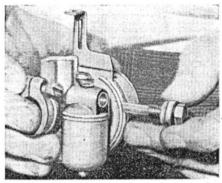
The wire gauze filter situated in the banjo union at the top of the float chamber is one of two precautions to prevent sediment from reaching the corburetter from the fuel tank. The second filter is located in the fuel tap inside the tank itself. Both should be brushed and washed regularly with petrol, and immediately inspected in the case of trouble.
