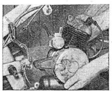
The three main stages in removing the engine: (top left) after removing the offside chain wheel, remove the lower engine bolt; (top right) loosen the upper engine bolt, but do not remove yet. Finally disconnect electric cables, fuel pipe and carburetter before removing upper bolt completely and lifting engine out of frame (lower left).
