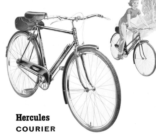
Frame: 19 in., 21 in. and 23 in. Wheels: 26 in.  $\times$  1 $\frac{3}{8}$  in., Endrick rims. Tyres: Dunlop Sports. Handlebar: All-rounder Bend on adjustable stem. Brakes: Caliper. Mudguards: Steel Spearpoint. Saddle: Spring seat. Pedals: Rubber. Accessories: Reflector, Inflator, Hold-all Bag and Spanners. Finish: Standard Black enamel, Carmine Red or Lincoln Green.
