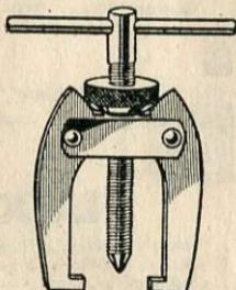
The safe way of removing difficult sprockets is to use these well made tools which should have a place in every handyman's garage. Two leg pattern for removing sprockets from confined places, as illustrated.
