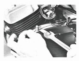
Disconnect the starting cable using a 17 mm (.669'') open end wrench as illustrated.
