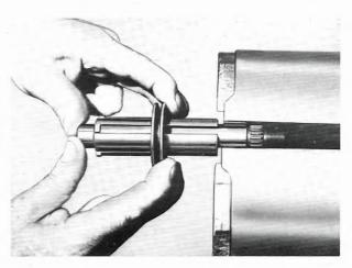
Secure in a vice the secondary shaft of the 5 speed engine, draw back and slide off the slider taking care not to lose the springs and locating balls.
