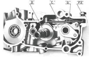
Fit the gearchange lever «C» slipping the gears operating slider into the sleeve «D» placed on the secondary shaft.
