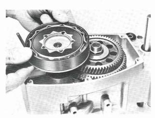
Remove with the screwdriver the pressure plate from the 4 rubbers.
