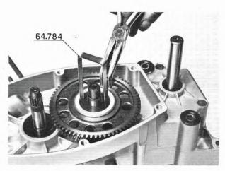
Remove the 2nd speed gear and then the 1st', while holding the catches with the tool 64784. Then slide the clutch hub and washers.
