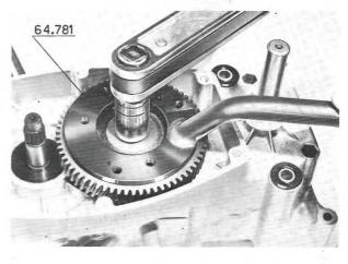
Fit the clutch assembly and hub following the illustration.
