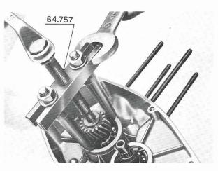
Hold the gear with the tool 64.757 operate its centre screw and slide the gear from the crankshaft with a 19 mm (.748'') wrench.
