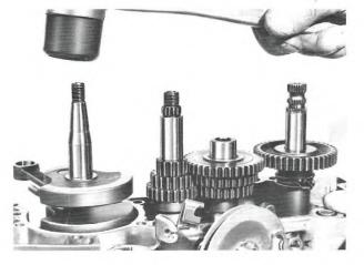
Slide the crankshaft, lightly tapping it with a mallet.
