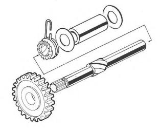
Mount the distance piece, the shaft, the engagement for starting with gear as shown in the illustration.
