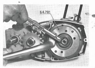
When satisfied that the gap is set correctly, fit the washer and tighten the fastening nut, using the tool 64781 and the 14 mm (.551'') socket previously used when dismantling.
