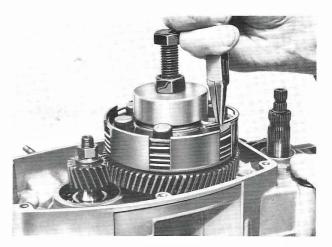
With the pliers remove the circlip, the spring plate and the clutch discs.
