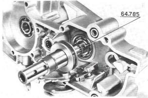
Mount the pin «P», the spring «M» and the gears locating lever, screw but do not tighten the locknut.
