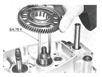
Place gears and freewheel on the primary shaft as per illustration. Use the tool 64784 to hold in place springs and catches when sliding the 1st speed gear.
