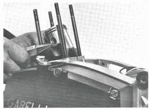
Check that the crankcase upper face and the cylinder base are clean and free from burrs. Lightly grease a new gasket on both sides and lay it on the crankcase face. Oil the cylinder bore and the piston skirt.
