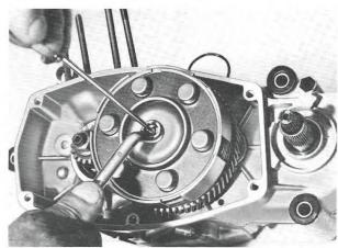
Grease the bore of the small end and the 21 needles 2 x 11,8, insert them in the small end eye holding them in place with the drift pin bush 64759.
