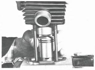
Check that the top of the cylinder and the face of the head are clean and undamaged. Fit the head over the studs and place the 4 washers and nuts on the studs. Tighten the nuts gradually in a cross pattern. The final torque should be 1,5÷1,8 kpm (in.lb. 0,084÷0,10).
