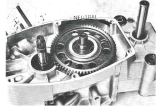
CAUTION: the freewheel hub shall be fitted so as to allow the 1st speed gear to turn free when rotated in the counter-clockwise direction.
