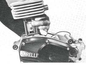
Check that the top of the cylinder and the face of the head are clean and undamaged. Fit the gasket and the studs and place the 4 washers and nuts on the studs. Tighten the nuts gradually in a cross pattern.
