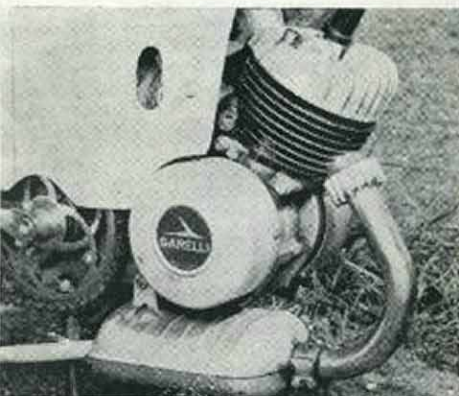
Heart of the Garelli moped is the 49cc two-stroke engine with its large efficient silencer and angled outlet.
