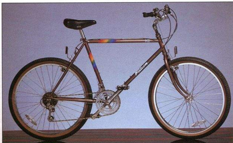
K2 A true all-terrain bicycle, with top quality components and performance to match. It's 18 speed gears will transport you over most kinds of terrain in comfort and style that our competition will find hard to match. SIZES: 21", 23". COLOUR: Metallic brown.
