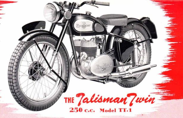
FRONT FORKS. Excelsior design TELESCOPIC Built with heavy gauge alloy steel tubing. Dual double action coil springs absorb all road shocks and provide perfect control under all conditions. Deep phosphor bronze bushes support the sliding members protected by double oil seals.
