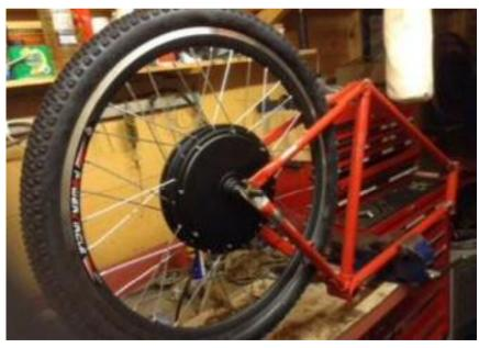
Dry fitting of the Electric motor wheel prior to going to the paint shop.
