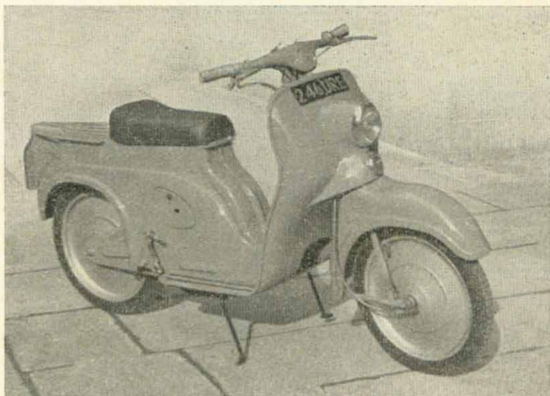
Conventional scooter lines combine with smooth and easy-to-clean exterior. Note disc type wheels.
