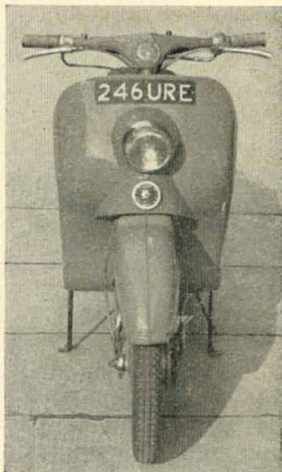
This front view shows good weather shielding and wide centre stand.
