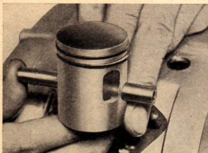
Fig. 25 Pressing gudgeon pin out of the piston
